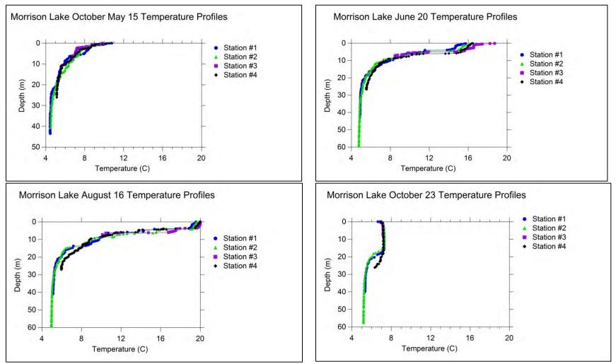
Figure 21 Temperature profiles from all Stations shown by date.
