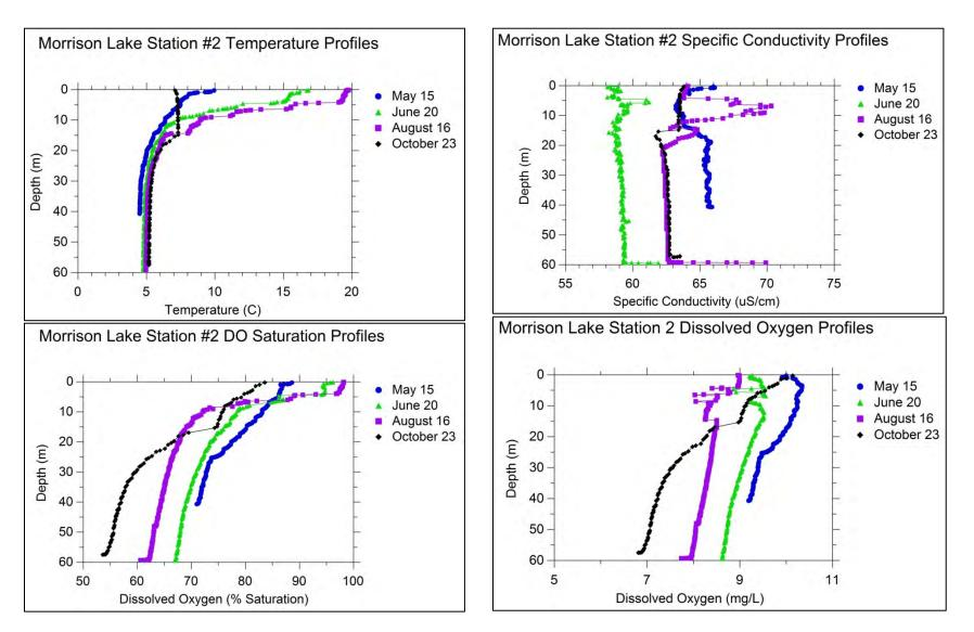
Figure 26 Temperature, conductivity and dissolved oxygen profiles at Station #2.
