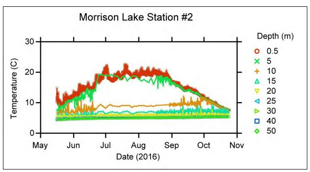
Figure 11 Temperature data from Station #2 thermistor chain.
